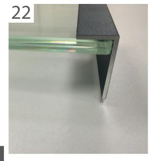
Glass roofs come with an angle iron, which is attached to the front of the glass pane. The angle iron is then sealed with sealant.
