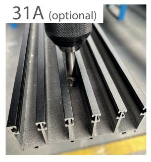
When placing an INVIGO PRO under the gutter, it must first be pre-drilled using a 4.2 mm diameter drill bit. Repeat this every meter, countersinking the holes.
