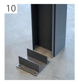
Remove the front part of the post. Place any included base plates on the foundation. Screw the posts to the base plate from the inside.
