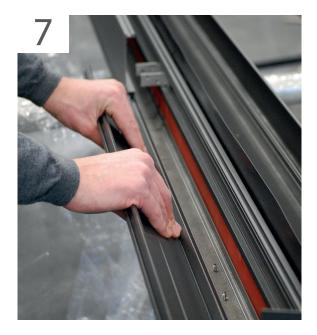
Release the gutter risers from the gutter by pulling them toward you. Install the bracket at a distance of 55 mm from the side of the gutter. Install the brackets at both ends of the gutter.
